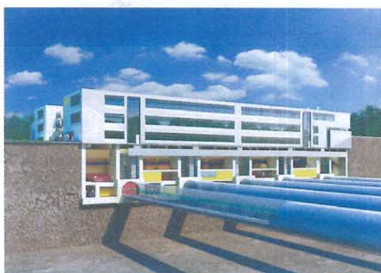
Fig. 1 Main building of the European XFEL. Five tunnels with a clear diameter of 4.60 meters lead to the underground experiment hall.
